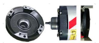
By adopting anti-dust-double-filter, we succeeded in preventing the mortar invading into the core of a motor. Moreover, by innovating enhanced exhaust port, we succeeded in redusing an operation sound to 5dB.
