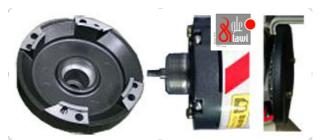
Adhered concrete is easily removed since the bearing case and inlet portion are fluorine coated. An exhaust port configuration is simply designed which enables maintenance easier. Moreover an inlet-port part equipped with double filter configuration of high dust proof, prevents mortar come into vibrator's inside.
